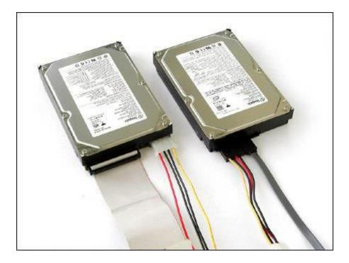
SATA (right) and IDE (left) hard drives. The SATA hard drive has the data cable on the right and power cable on the left. The IDE data cable is ribbon-like (on the left)
